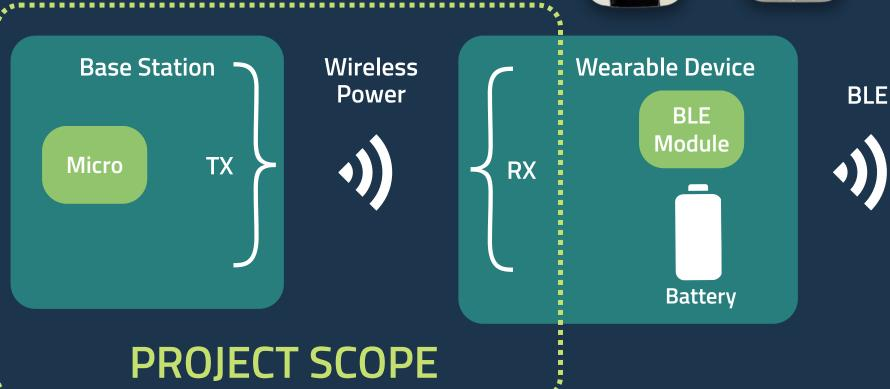
Our wireless charging platform uses a base station powered via USB to transmit energy wirelessly through a TX coil. The wearable device receives this power through an RX coil, storing it in a battery while enabling communication via a Bluetooth Low Energy (BLE) module.
